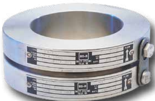
BS&B Quik-Sert safety head - flanges are assembled with bolted side lugs in sizes through 8 inches ID - with recessed cap screws in 10 inch size and up
